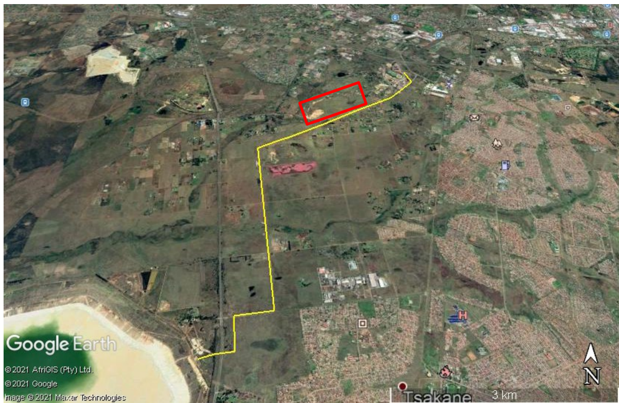
Figure 3: Google Earth map to show the proposed routes (yellow) for the overhead power lines for the Tshedza 1 PV plant.
